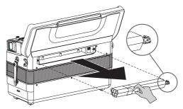
The battery is connected to the FR-7/FR-5 by means of a cable. You need to disconnect the cable from the battery by pressing the clip on the connector before fully removing the battery.
